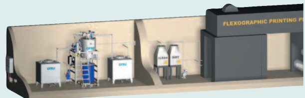
Concept OFRU solvent distillation unit ASC-150, direct connect to a printing machine.
