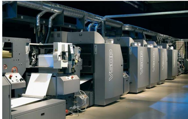
**Variable Sleeve Offset Printing (VSOP) Rollenoffset-Druckmaschine.**
