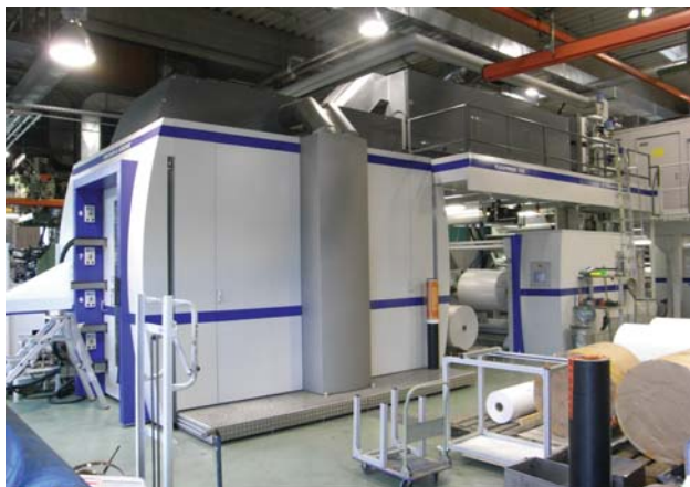
Right: Each day, the ASC-150 solvent recovery plant installed at Debatin distils 250 l of soiled solvent.
